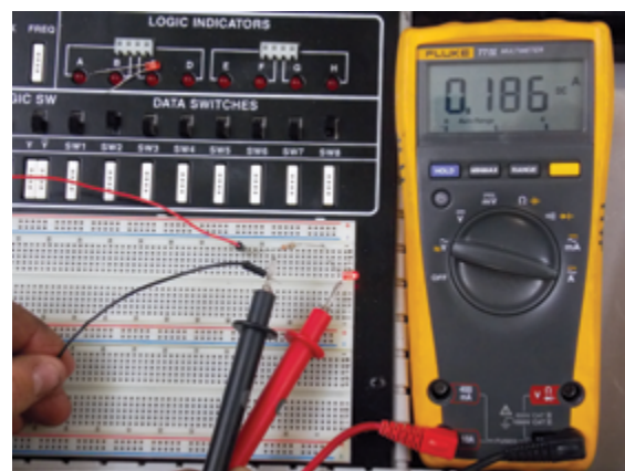
Figure 2.5 Using a volt meter to test current (courtesy author)
