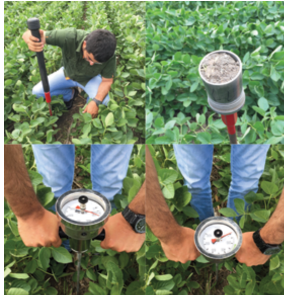
Figure 14.2 Measuring the bulk density (top images) and soil resistance (bottom images) in a field. (Courtesy of the authors)
