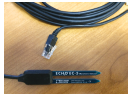
Figure 33.7. ECHO EC-5 soil water content sensor (Decagon Devices, Pullman, WA, Decagon.com). Note the RD-45 connector at the end of the cable for easy connection to a data logger. (Courtesy of Todd Trooien, South Dakota State University)
