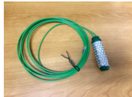
Figure 33.6 Watermark® Granular Matrix sensor. (Irrometer, Co., Riverside, CA). (Courtesy of Todd Trooien, South Dakota State University)
