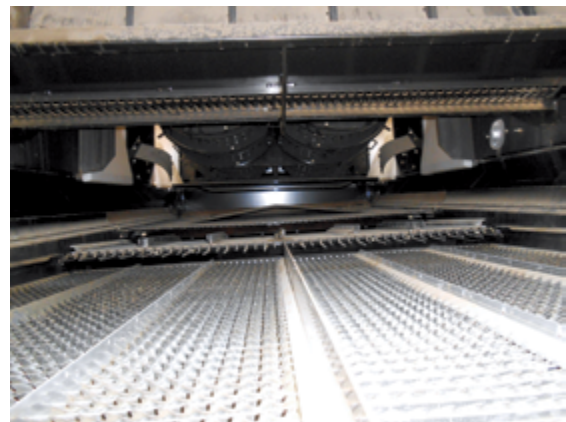
Figure 37.4 The sieve elements that collectively make up the cleaning shoe. Most common adjustments involve adjusting fan speed and sieve openings to regulate the flow of grain through the shoe and the movement of chaff to the rear.
