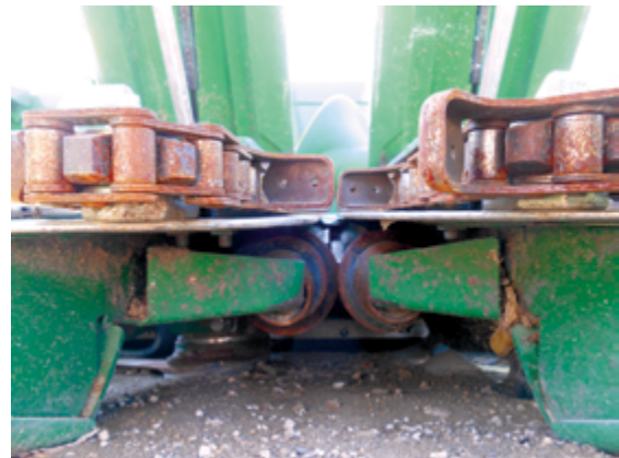
Figure 37.2 Position of snap rolls, deck plates, and gathering chains. Deck plate spacing is typically narrower where stalks enter and the gap is centered between snap rolls. Gathering chain lugs should extend about 1/4” into the deck plate gap.
