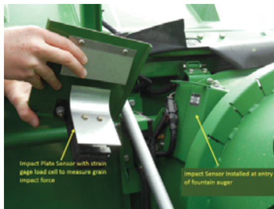
Figure 50.1 An impact-style flow-rate sensor using a curved plate and strain gage load cell to measure impact force of grain. The sensor is installed at the base of the fountain auger where grain leaving the clean grain elevator impacts. (Courtesy of authors)
